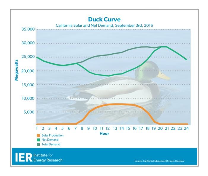
In the graph, we can clearly see what is known as the "duck curve" in the industry. The duck curve, named for its similarity to a duck's silhouette, shows the disruptive effect increased levels of solar penetration have on grid operation.
